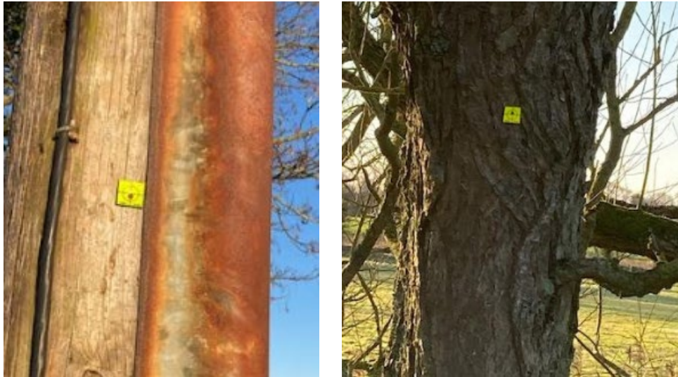
Figure 17: Telegraph pole and tree with yellow targets used in total station coordinate reference work.
