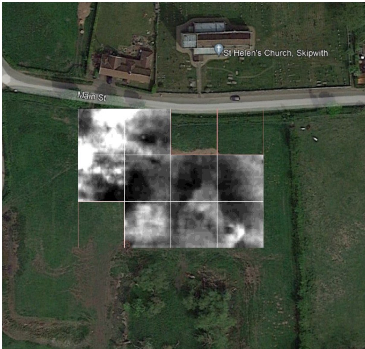
Figure 22: Survey area overlaid onto aerial image. Grid squares are 20m x 20m.
