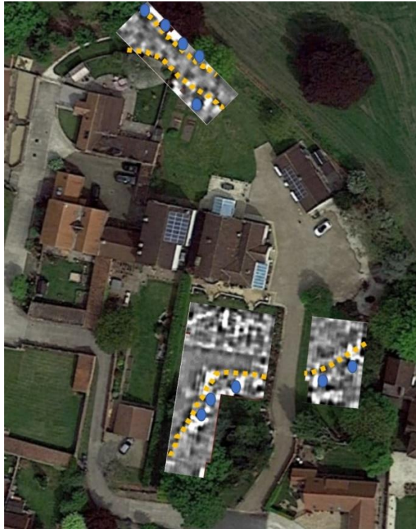
Figure 33. Geophysical survey showing the course of paths and tracks running north and south of the house. Tracks are marked in yellow dotted lines and the trees are the blue circles.
